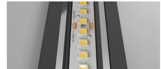
The shape of the cable allows the installation of a LED strip [optional 13W/m, 48V maximum width 10mm] for indirect lighting. The light emission of the LED strip enlightens the cable in its transparent version. The 48V LED strip has an IP54 degree of protection, obtained through protection with nano technologies for best lumen yield and best color rendering.
