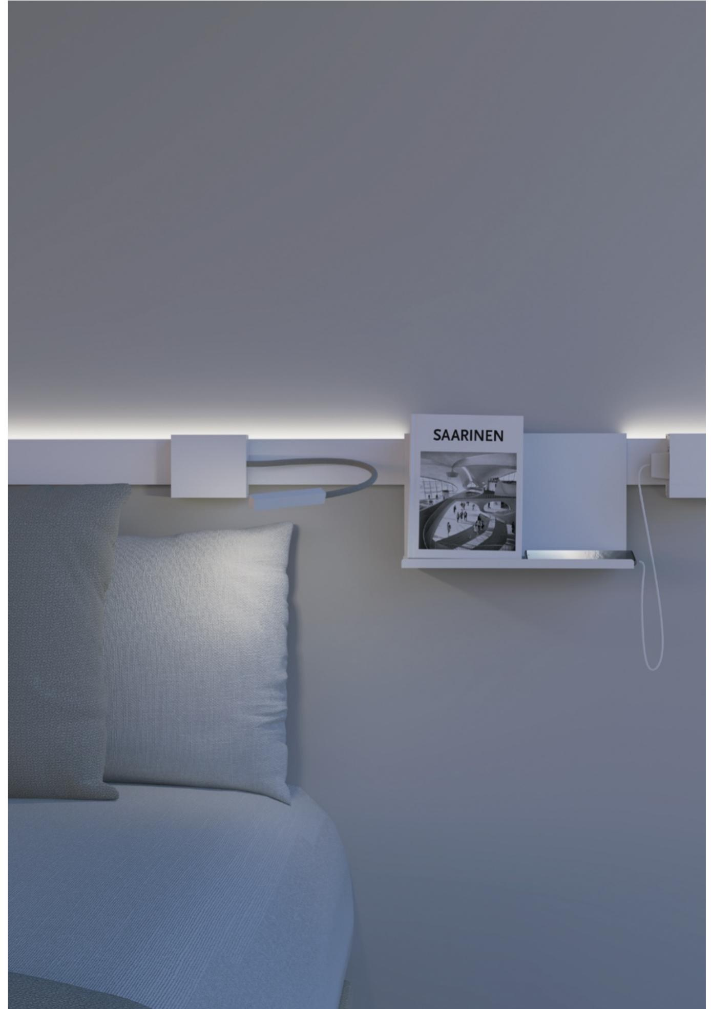
NUO is a reading light with a diffuser designed to avoid glare. NUO is available in the left and right version. LED lighting device with a flexible arm covered in anthracite grey fabric. Anodized aluminium structure and dissipater. Integrated Shuttle device [enables the connection to the selected power line of the track]. Touch switch for switching on and LED circuit diffraction. Integrated power supply.
