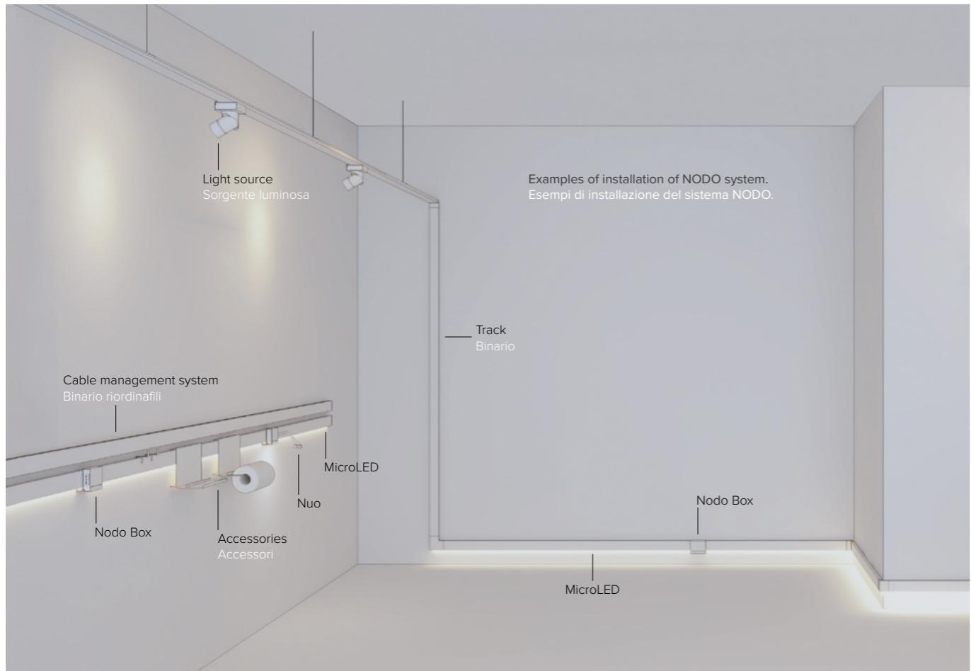
Electrical copper conductors inserted in a profile of insulating material [glow wire 850°]. With a single-phase AC connection, the maximum load is 16A [3840W]. The 3-phase version of NODO track, if connected to 3-phase alternating current, allows a maximum load of 16A per phase [3 x 3840W = 11520W]. The track has grooves that enable anti-glare installation of 8 mm LED strips on both sides [Side Light] and LED strip up to 20 mm on the back [Up Light] if suspended.
