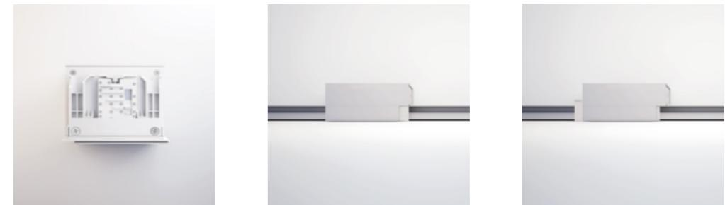
The Shuttle slide device is operated with a simple gesture that makes the mechanical coupling of the socket and light elements to the track and their electrical power supply possible at the same time. The integrated phase selection switch lets you choose which of the 3 lines on the track to connect each element.
