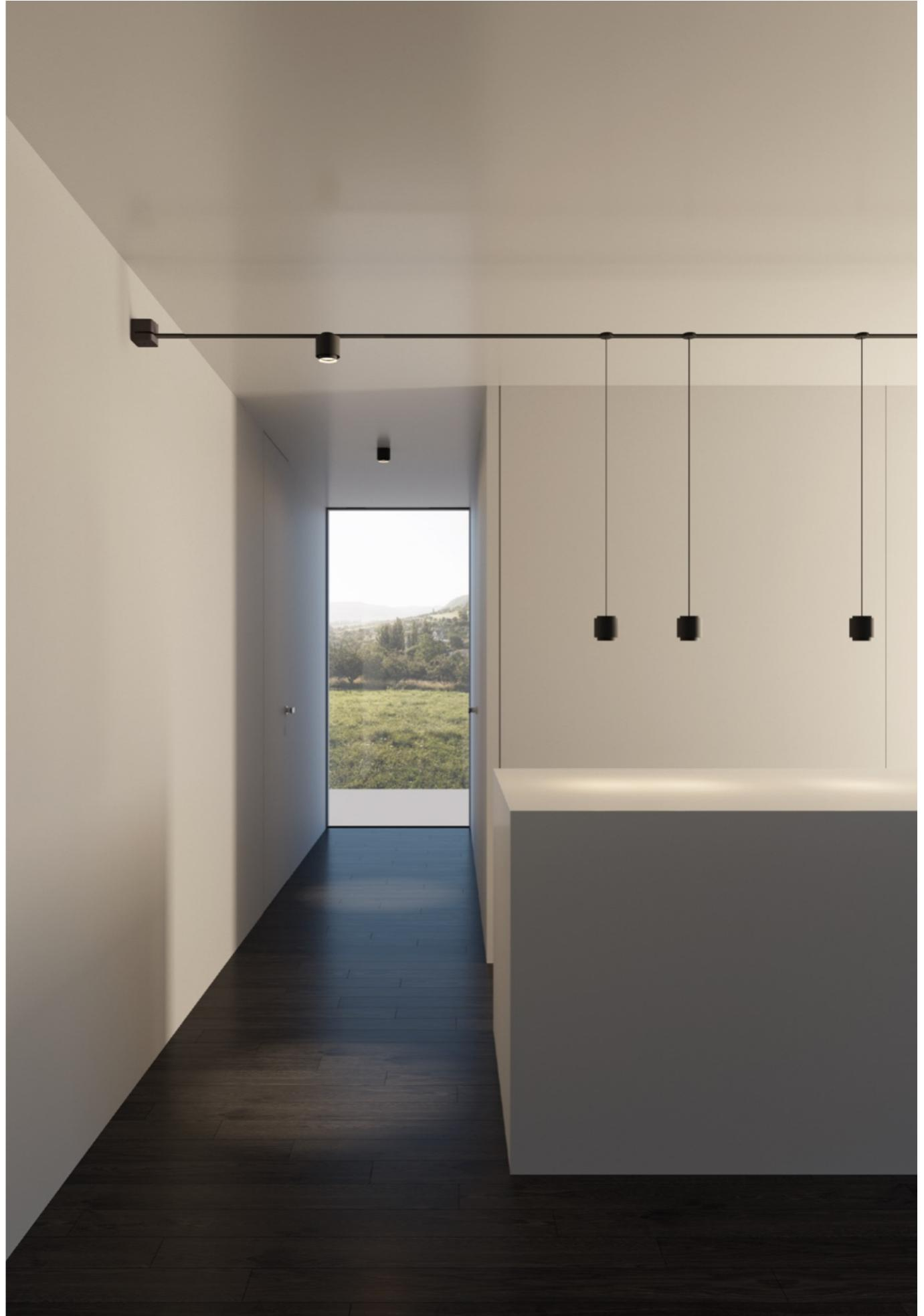
ZOOM sources can be connected to other types of systems [DALI, Insulated pushbutton, Potentiometer Linear 100K, 0-10V Passive, 1-10V Passive]. In the ONE BY ONE dimmable version the sources can be controlled separately (DALI), in the PWM dimmable version they are all controlled together. Rotating optic [patent pending] allows endless beams from 12 to 46 degrees.
